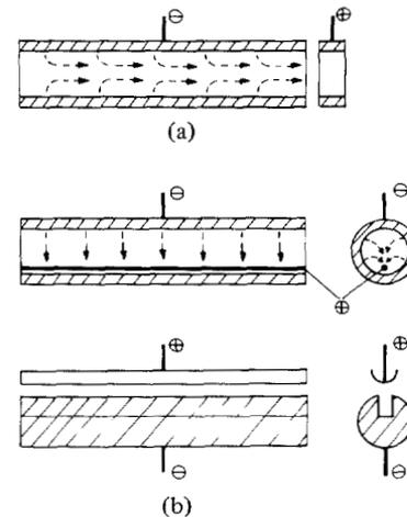
Fig. 1. Illustration of (a) longitudinal and (b) transverse (inner-anode and slotted type) HCD.
