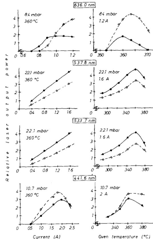
Fig. 3. The dependence of He-Cd<sup>+</sup> laser power on the discharge current and oven temperature for the longitudinal (broken line) and transverse HCD. Single-line operation.
