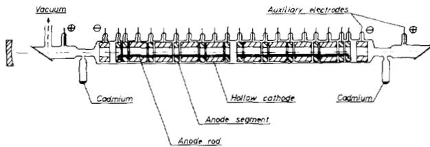
Fig. 2. Tube structure of He-Cd<sup>+</sup> laser with longitudinal and transverse HCD.
