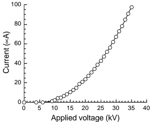
Fig. 3. Corona current as a function of applied voltage.
