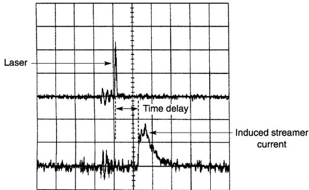
Fig. 5. Time relationship between laser and induced streamer (laser sheet:  $h = 30$  mm,  $d = 10$  mm, laser energy density = ca.  $3.3$  mJ/cm<sup>2</sup>, applied voltage = 25 kV, 200 ns/div., current = 20 mA/div.).
