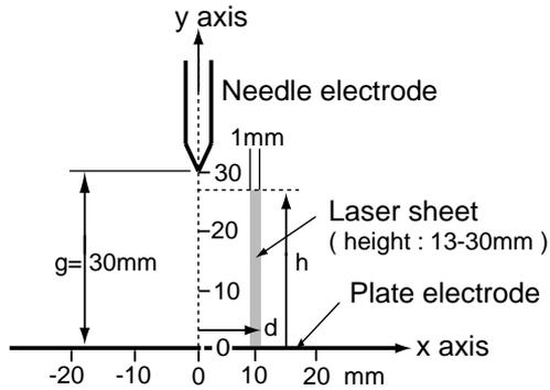
Fig. 2. Definition of the laser sheet position.
