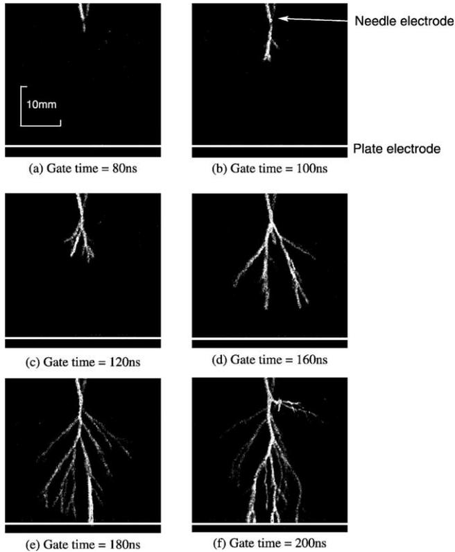
Fig. 7. Characteristics of laser-induced streamer discharge (laser sheet:  $h = 30$  mm,  $d = 2$  mm, laser energy density = ca.  $3.3\text{mJ}/\text{cm}^2$ , applied voltage =  $25$  kV).
