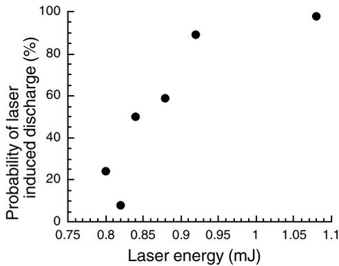
Fig. 4. The probability of the laser-induced discharge as a function of incident laser energy (laser sheet:  $h = 30$  mm,  $d = 0$  mm, applied voltage = 25 kV).
