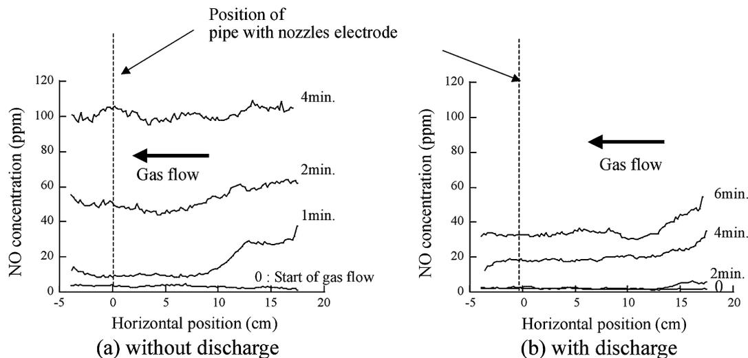
Fig. 7. Spatial NO distribution for various operating times after NO mixture gas supply. (a) Without discharge. (b) With discharge (27 kV, 83  $\mu$ A). Treatment gas: NO(100 ppm)/air, 3 L/min, Injection gas: mixture of air(0.4 L/min) and CO<sub>2</sub> (40 mL/min).
