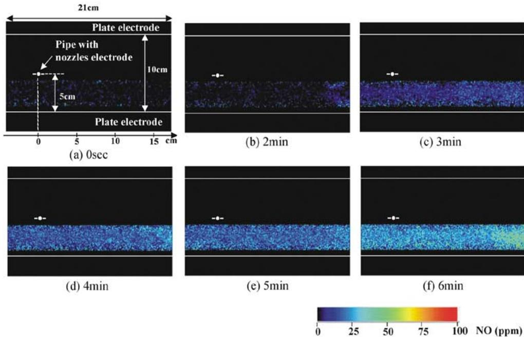
Fig. 6. Wide-range 2-D NO concentration profiles under the discharge condition (27 kV, 83  $\mu$ A) as a function of time after NO mixture gas supply.
