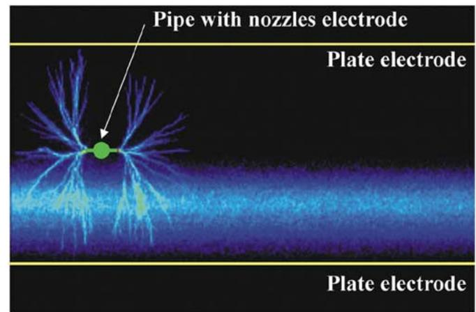
Fig. 3. Simultaneous recording of NO LIF signal and light emitted by the laser-induced streamer. Applied voltage: 27 kV, NO/air 3 L/min. Gate width of ICCD: 490 ns for capturing both the NO LIF signal and the light emitted by the induced streamer corona.
