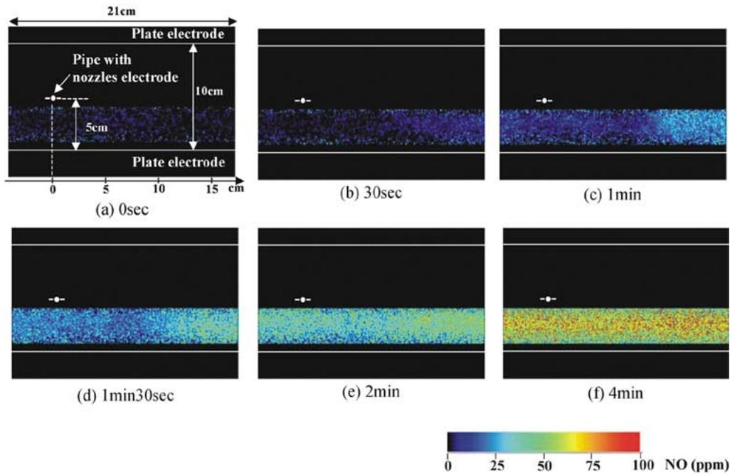
Fig. 5. Wide range 2-D NO concentration profiles under the nondischarge condition as a function of time after NO mixture gas supply.
