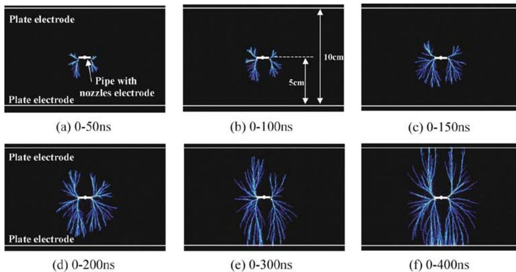
Fig. 4. Images of the streamers induced by a single laser pulse for various exposure times of the ICCD camera. Streamer inception time represented by “0”ns was determined by adjusting the gate time of the ICCD camera. NO(100 ppm)/Air, 3 L/min. Applied voltage: 30 kV. Corona current: 134  $\mu$ A.
