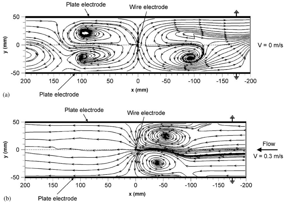
Fig. 2. Flow streamlines in the wire-to-plate type ESP. The primary flow velocities: (a) 0 m/s ( $Re = 0$ ), (b) 0.3 m/s ( $Re = 2000$ ). Positive voltage varied from 30 to 32 kV to maintain discharge current at  $150 \mu\text{A}$  ( $E_{hd} = 2 \times 10^8$ ).
