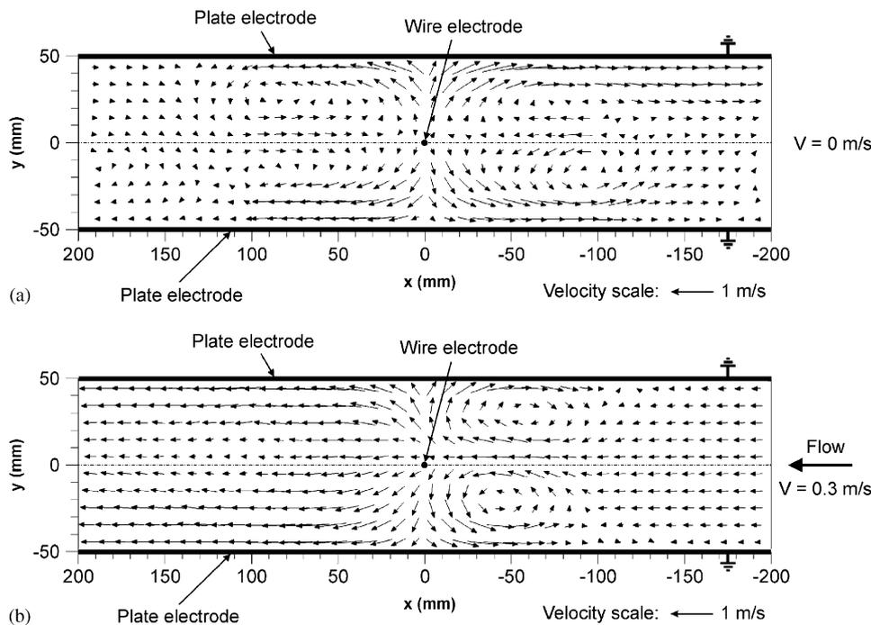
Fig. 1. Flow velocity field patterns in the wire-to-plate type ESP. The primary flow velocities: (a) 0 m/s ( $Re = 0$ ), (b) 0.3 m/s ( $Re = 2000$ ). Positive voltage varied from 30 to 32 kV to maintain discharge current at  $150 \mu\text{A}$  ( $Ehd = 2 \times 10^8$ ).
